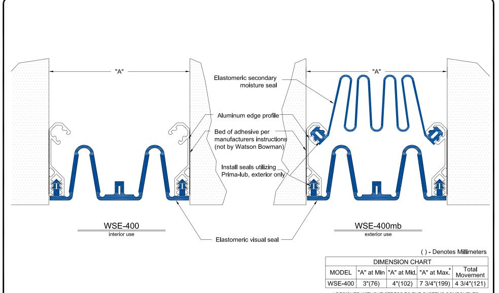
\* DESIGNED WITHOUT STRESS TO THE SYSTEMS COMPONENTS. CAPABLE OF WIDER OPENINGS DURING SEISMIC EVENT.
